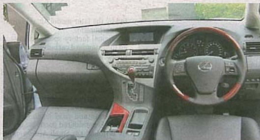
Dashboard is divided into an upper display screen and lower operation zone. Missing in the local spec is the i-Drive-like controller.
